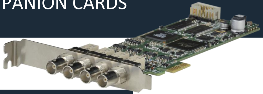
A-LTC-CARD-1 mounted on DELTA-3G-elp(-d) 40, DELTA-hd-elp-d 80, DELTA-hd-elp-d 62 or DELTA-hd-elp-d 44
