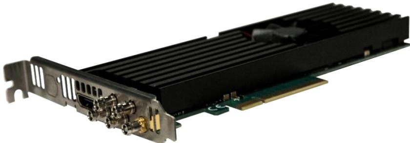
The DELTACAST Mixed Interfaces cards are designed for easy integration with customer applications. A comprehensive software development kit (SDK) includes device drivers for standard platforms, a range of ASI and SDI processing services and an easy-to-use programming interface for controlling the card.
