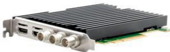
The DELTACAST Mixed Interfaces cards are designed for easy integration with customer applications. A comprehensive software development kit (SDK) includes device drivers for standard platforms, a range of HDMI and SDI processing services and an easy-to-use programming interface for controlling the card.
